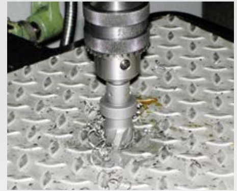
Bohren in Riffelblech
