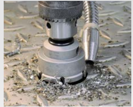
Bohren in Riffelblech
