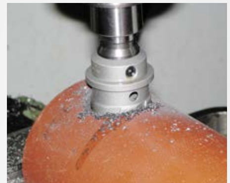
Bohren in Rohre
